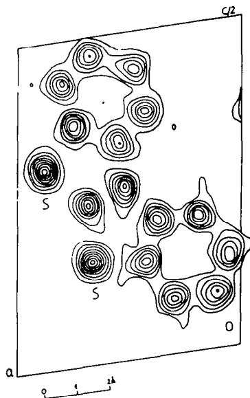
FIG. 1 [1]Benzothieno[2,3- b ]benzothiophene. Electron density projection along the b axis based on the h 0 l structure factors. Contours at intervals of 1 electron/Å 2 for the carbon atom and at intervals of 3 electrons/Å 2 for sulfur. The first contour represents 1 electron/Å 2 .
